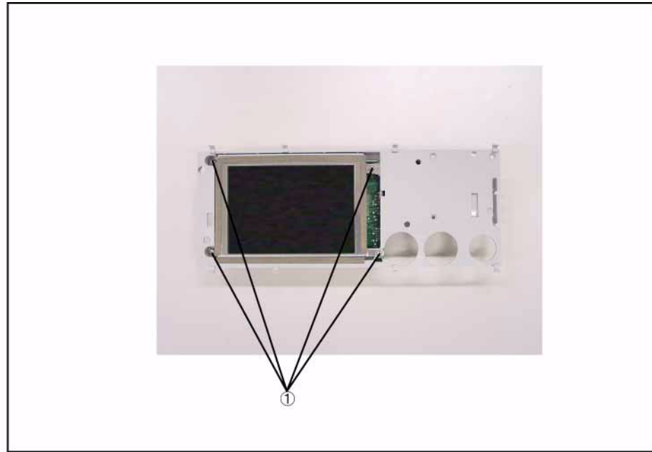
Figure 6-22 LCD and Display Interface Board Replacement
